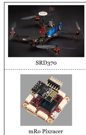
Figure 4.5.1: Quadrotor srd370 frame and associated mRo Pixracer
