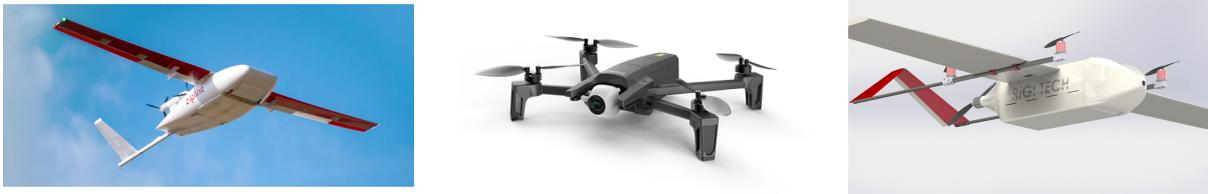
Figure 1.0.2: From left to right, an example of Fixed wings drones (ZipLine), multicopters (Parrot) and VTOL drones (Rigitech)
