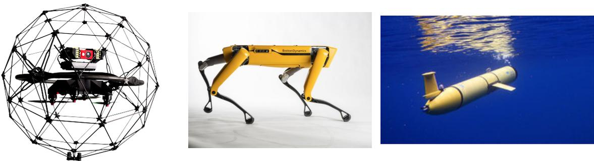
Figure 1.0.1: From left to right, an example of UAV (Flyability), UGV (BostonDynamics) and UUV (Maracoos)
