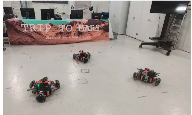
Fig. 1. Formation with 3 agents. The formation is defined as relative positions and attitudes with respect to the camera frames, which can be translated into the agent’s frames.
